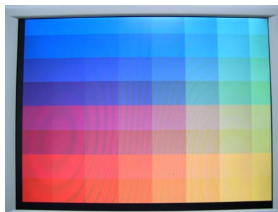
Figure 2.3. The default VGA output pattern when SW0 is set to DOWN position.
